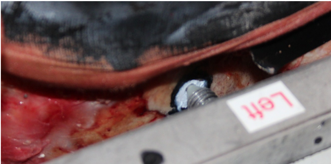
Figure 4.16. Divot at center of curvature aligned with the fixture axis of rotation using positioning pointers.
